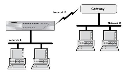
Note that even though network segment B uses two modems to transfer data rather than a physical cable, it looks like a cabling segment to Network A and Network C.
